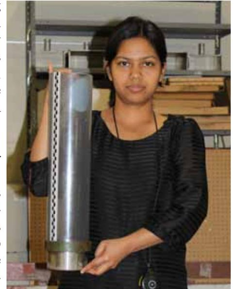
FIGURE 1: Modified Philip Dunne Infiltrrometer (Courtesy F. Ahmed)
